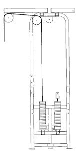
Figure 19. Tricep pushdown cable routing.
